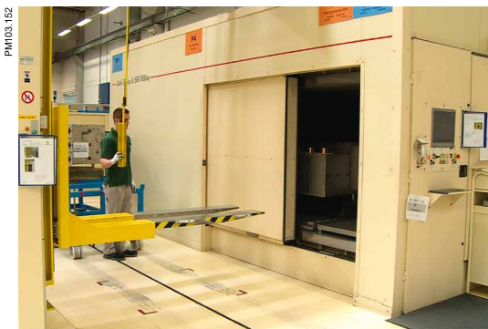
Integral routine leakage test
